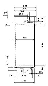
Electrical inlet (power) Refriaerant Inlet Refrigerant Outlet
